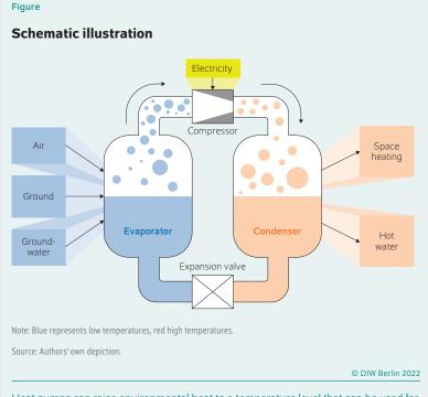
Heat pumps can raise environmental heat to a temperature level that can be used for space heating.
